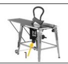
• Connect the hose of the extraction system to the funnel of the machine (1). The necessary information can be found in the Technical data chapter.
