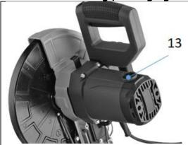
Check the carbon brushes after the first 50 hours of operation with a new machine or when new brushes are installed. After performing the first check, repeat the check every 10 operating hours.
