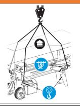
When using a crane for lifting (e.g. when loading the splitter onto a truck), attach the hoist only to the intended places - see illustration on the left.
