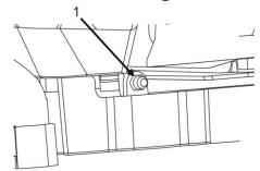
The gearbox is lubricated at the time of delivery of the machine, but must be relubricated at regular intervals (see maintenance schedule).
