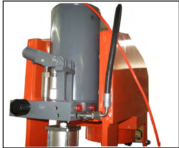
Fig. 13: Mount the short hose
