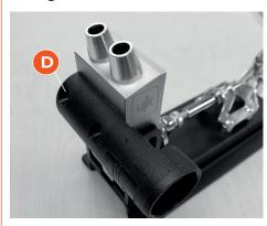
Locate the dust extractor assembly and the two Hex screws **(D)**. Line up the pre-drilled holes with the threaded holes to the front of the guide block and secure with the two Hex screws.
