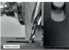
Step 3 Select the pilot drill tip to suit the timber thickness (see Drill guide chart). Place the ring collar clamp (C) on to the drill bit shaft, inset the drill bit into the bushing guide hole, lower the drill bit so it's 2-3mm below the base plate and tighten the ring collar flush against the bushing guide. DO NOT OVERTIGHTEN!
