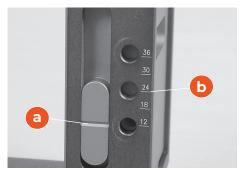
Step 2 Line-up the machined groove (a) with the numbered scale (b) to match the timber thickness. See the "Drill Guide Block Chart" to set the correct height. Lock the block in position using the two threaded locking pins (c).
