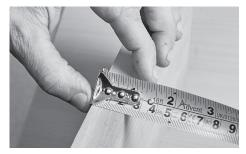
Step 1 Measure the width of the timber, see picture above.
