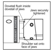
Always ensure that all faces are clean prior to fitting. Check the dovetail of the Wobble Chuck is flush inside the dovetail of the jaws and the shoulder is seated onto the face of the jaws. Then close the jaws tightly to secure the Wobble Chuck in place.
