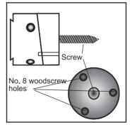
There are two ways of securing a workpiece with the Wobble Chuck. Firstly there is a screw which is ideal for quick and easy fixing. Alternatively there are three holes which enable fixing by No.8 woodscrews for larger projects.
