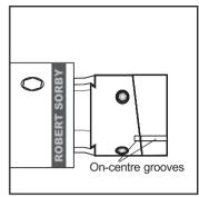
When the grooves of the Wobble Chuck are in-line the chuck is oncentre. To adjust the position of the grooves slacken the two screws in the bottom section turn the top section to the required postion and then retighten the screws.
