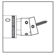
When using the screw ensure the grub screw is tightened into position. If using No.8 woodscrews without the screw, always remove the grub screw to prevent loss.
