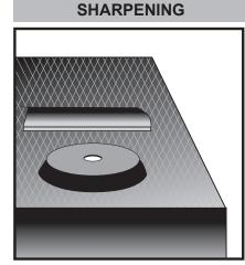
Both tips can be sharpened using a flat sharpening stone or a diamond file (ref RS224). For the perfect sharp edge use the cutter holder (ref 472) in conjunction with the Robert Sorby ProEdge (472 is not suitable for Midi Hollowmaster ref RS130KT).
