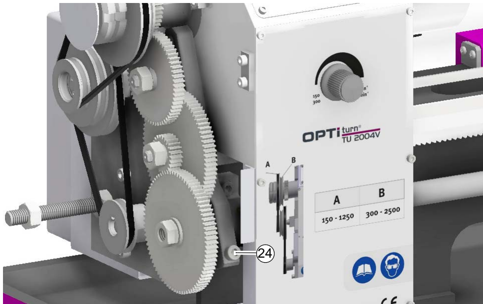
Img.4-9: Locking screw quadrant
