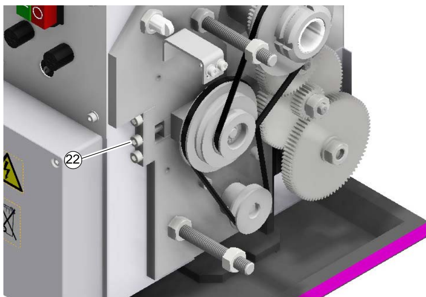
Img. 4-7: Synchronous belt position change
