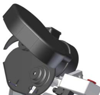
Img.3-7: Assembly V-belt housing
