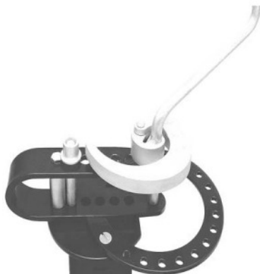
Fig. 37: Bending segments for spirals
