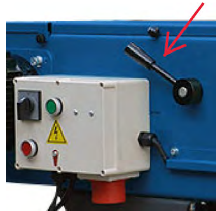
Fig. 13: Relaxing the sanding belt
