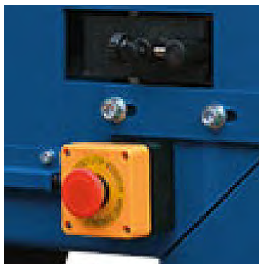
Fig. 3: Emergency stop button
