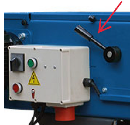
Fig. 11: Loosen the grinding belt
