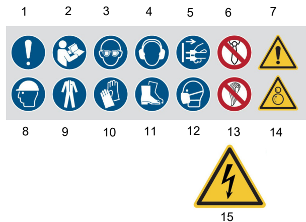
Fig. 1: Safety labels I1 General mandatory sign! | 2 Read the operating instructions! | 3 Wear eye protection! | 4 Wear ear protection! | 5 Pull out the main plug! | 6 Operation with tie forbidden | 7 general warning sign | 8 Wear head protection | 9 Wear protective clothing | 10 Wear hand protection | 11 Wear foot protection | 12 Wear a mask | 13 Operation with long hair forbidden | 14 Warning about rotating machine parts, danger of catching | 15 Danger high voltage.
