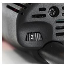
The speed can be infinitely adjusted to any application. In addition, the digital electronics are equipped with soft start, constant speed under load, idle speed reduction and overload protection.
