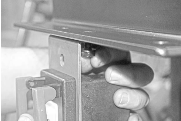
Mounting Control Switch with 2 longer hex bolts and flat washers
