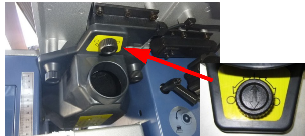
Fig. 17: Mounting the extraction device
