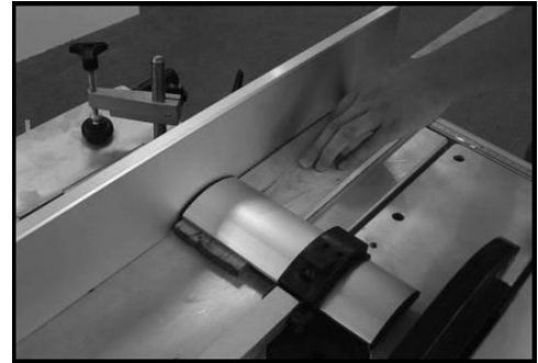
Fig. 34: Guide the workpiece to the stop
