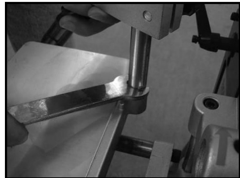
Fig. 12: Mounting the workpiece clamping device
