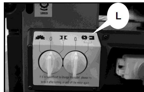
Fig. 30: Setting the planing function
