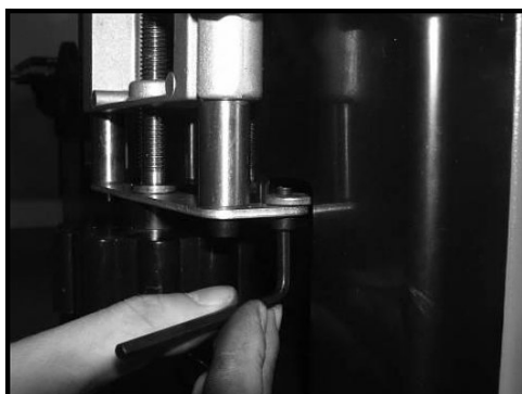
Fig. 11: Screw the milling table to the machine table
