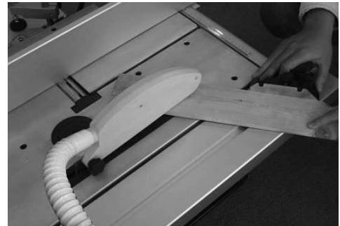
Fig. 24: Angle cut using the mitre fence
