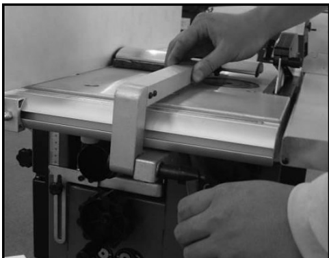
Fig. 33: Adjusting the stop
