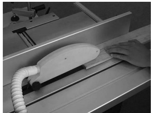
Fig. 23: Performing the cut
