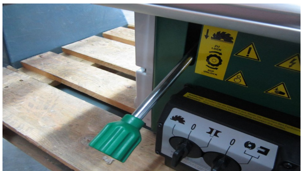
Fig. 46: Locking the saw blade
