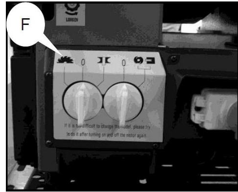
Fig. 16: Setting the sawing function
