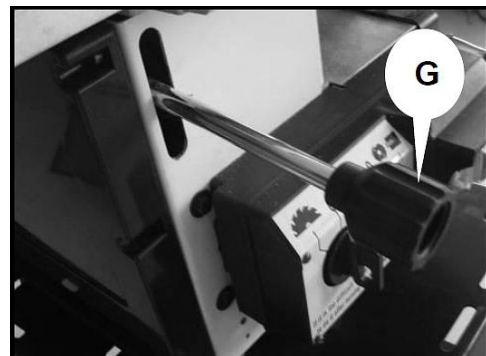
Fig. 18: Adjusting the position lever
