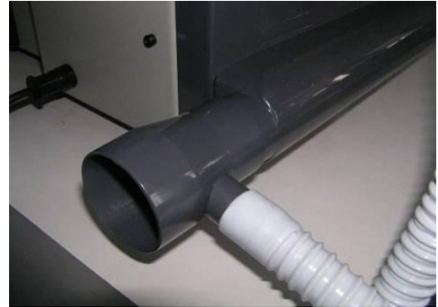
Fig. 22: Mounting the extraction hose on the extraction pipe
