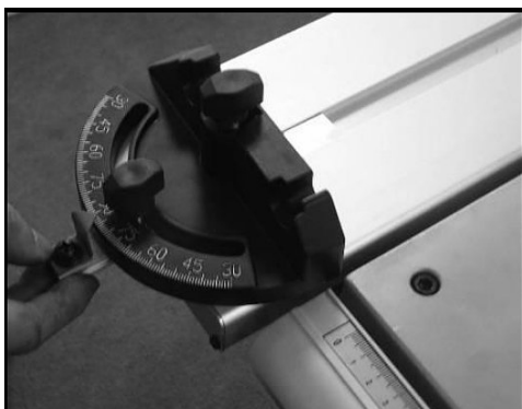
Fig. 9: Mounting the mitre fence
