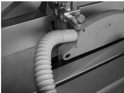
Fig. 21: Mounting the extraction hose
