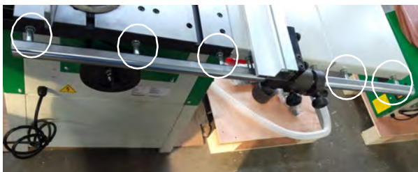
Fig. 8: Mount the stop guide rail
