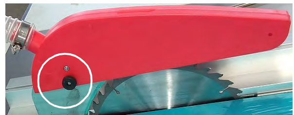
Fig. 16: Mount saw blade guard
