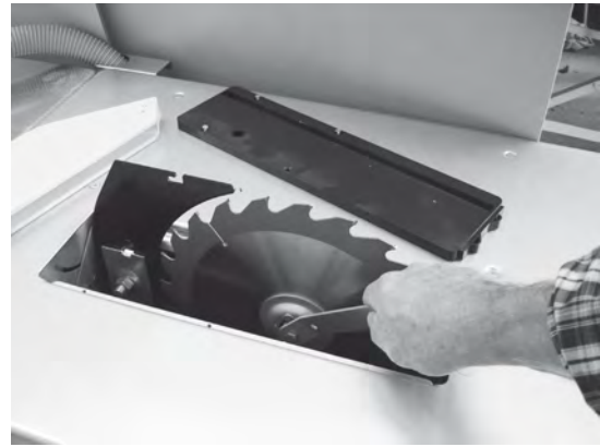
Fig. 39: Release the saw blade with the saw blade wrench
