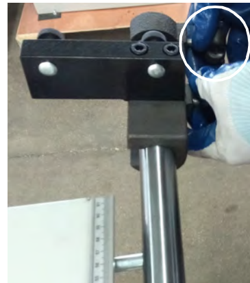
Fig. 9: Sliding the carrier onto the guide rail
