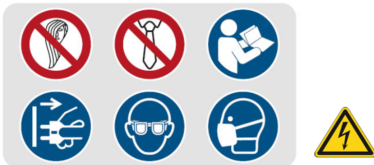
Fig.1-1: Safety signs - Prohibition signs: Operation with long hair prohibited, Operation with a tie prohibited | Mandatory signs: Observe instructions for use, unplug, wear eye protection, use respiratory protection | Warning signs: Warning of hand injury, Warning of electrical voltage
