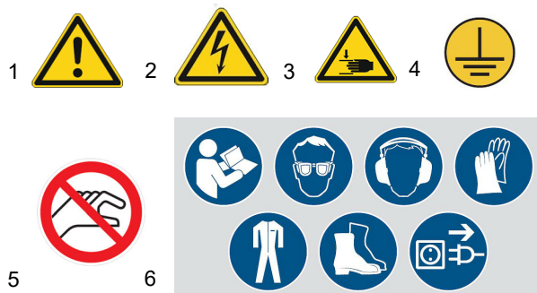
Fig. 1: Safety signs: 1 Warning of dangers | 2 Warning of dangerous electrical voltage | 3 Crushing hazard warning for upper limbs | 4 Ground symbol | 5 No Touching | 6 Safety instructions
