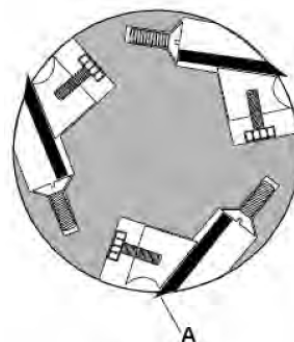
Fig. 17: Cutter head cross-section
