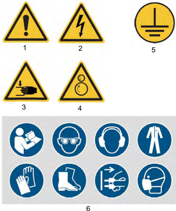
Fig. 1: Safety labels 1 Warning of danger | 2 Warning of dangerous electrical voltage | 3 Warning of hand injuries | 4 Warning of danger of entanglement | 5 Ground symbol | 6 Mandatory signs
