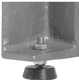
Fig. 7: Screw in machine feet
