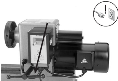
Fig. 18: Positioning of the headstock
