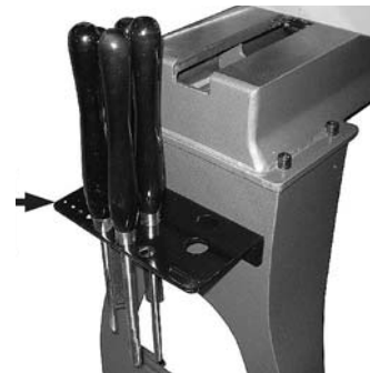
Fig. 9: Mounting the tool holder
