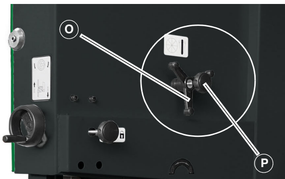
Fig. 20: Adjusting the saw band run
