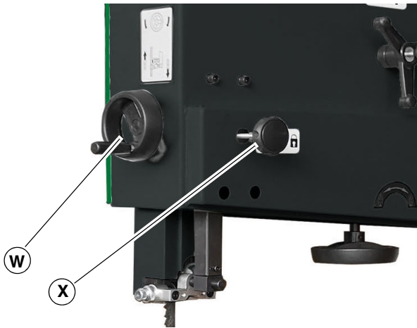
Fig. 26: Adjusting the position of the saw blade guide
