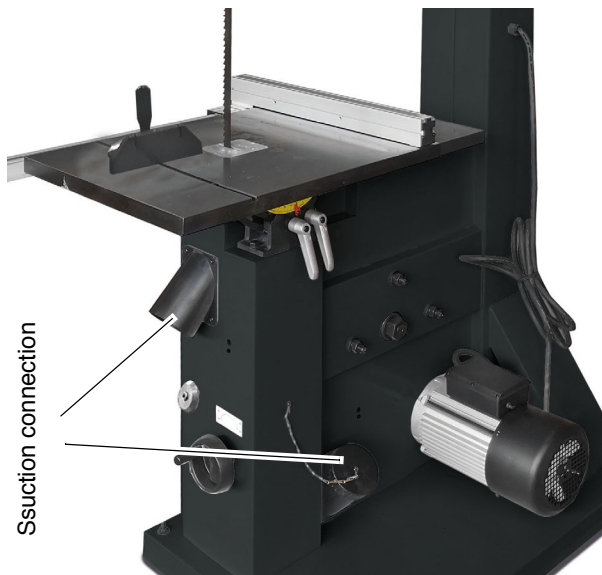
Fig. 15: Assembly of the suction hose
