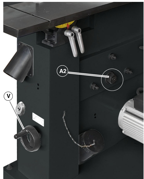
Fig. 32: Replace drive belt
