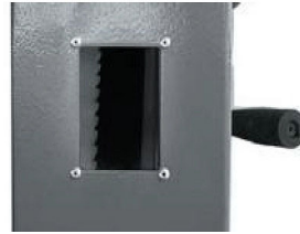
Fig. 21: Window saw band run
