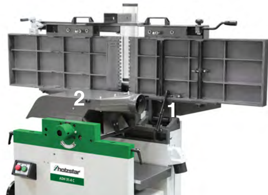
Fig. 9: conversion to thickness planing function
