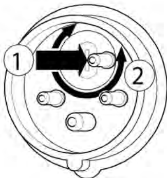
Fig. 5: Change motor direction of rotation
