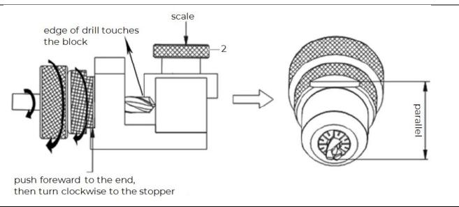
. Reset the scale ring: Turn the drill size adjustment knob (2) clockwise as far as it will go and then counterclockwise to the size of the drill (e.g. 8 mm).
