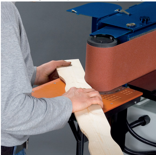
Fig.10-3: Grinding outer radii and arcs
