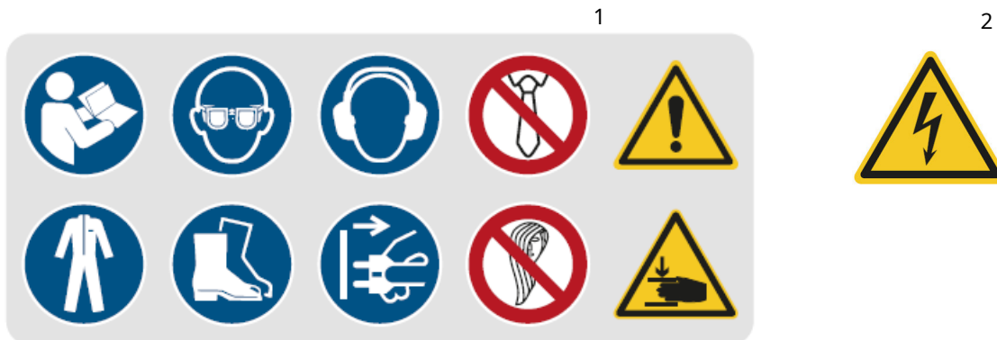
Fig.1-2: Safety signs - 1 mandatory sign: Observe instructions for use/operating instructions, wear protective clothing, wear eye protection, wear safety shoes, wear hearing protection, unplug before opening, operation with a tie prohibited, operation with long hair prohibited, warning of a hazardous area, warning of hand injuries 2 warning signs: Warning of electrical voltage
