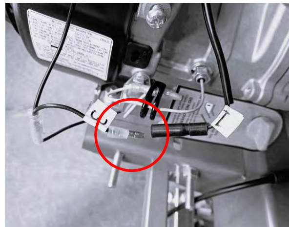
Step 2: Disconnect the black connection.
