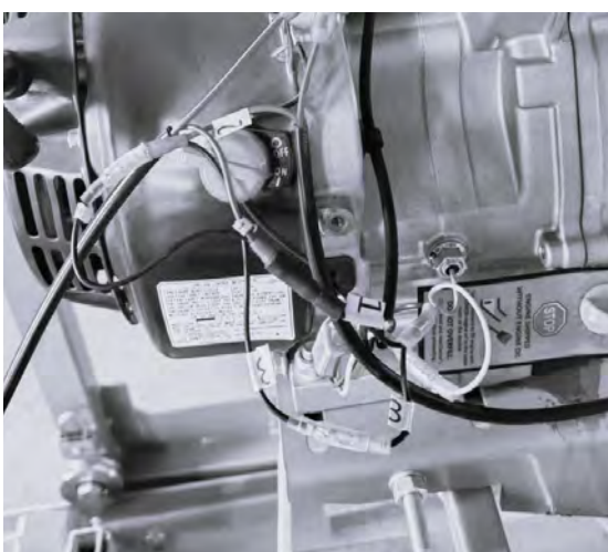
Step 5: Connect A1 and 1; Connect B3 and 3
