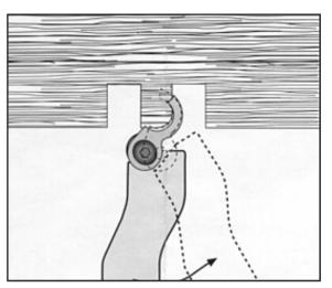
Now move the cutter as above and with just the fluted cutting edge cutting, gently sweep the tool so that the right hand side of the ring can be formed.
