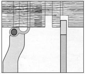
Adjust the cutter back as above and mark on the wood where the ring will be formed and then remove waste either side of the lines using a parting tool.
