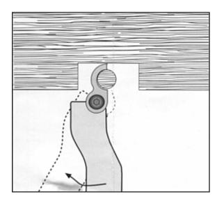
Remove the screw and cutter. Turn the tool over and replace the cutter so that it is facing right. Now repeat the previous 2 operations from the left side.
