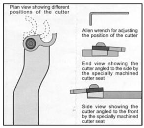
Included with the tool is one captive ring cutter, a machine screw and allen key/wrench.
