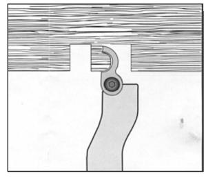
Adjust the cutter so that it is parallel with the shaft and finish the right hand side of the ring.
