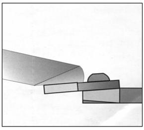
Sharpen across both the top and bottom face of the cutter using a honing stone or diamond file.
