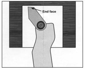
The box can be hollowed from the centre outwards using a gentle sweeping action. Adjust the cutter so that the end face cuts a flat bottom and neatly into the corner.
