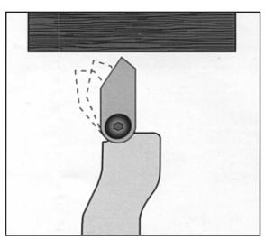
The cutter can be adjusted to suit the best position for the cut required. To start hollowing use the cutter in-line with the shaft and bore the centre of the box.
