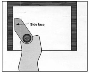
Adjust the cutter back so the side face is flat to create parallel sides to the box.
