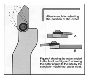
The Box Hollower is fitted with the side/end box hollowing cutter and comes with an Allen key/ wrench for cutter adjustment.
