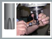
Chamfered tool tips eliminate burrs and help tools seat in screw head
