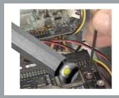
ProHold® buttons are non-magnetic and safe for use in electronic applications and with nonferous (brass, stainless, plastic, aluminum) fasteners
