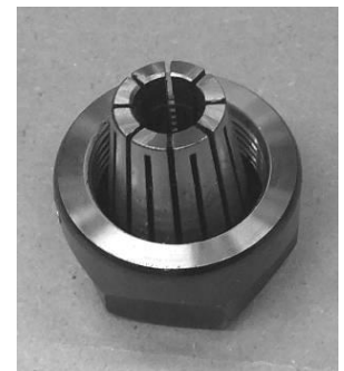
Collet fitted to Spindle Nut
