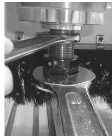
Collet fitted to Spindle Nut
