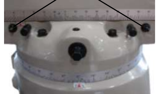
Ram gib adjustment screws
