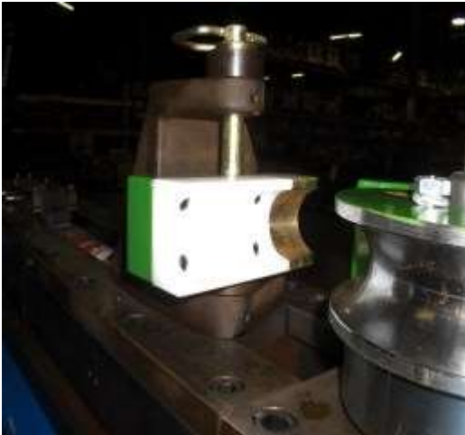
Installing counterdie with 3/4" pin
