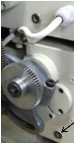
Gearbox Oil Drain
