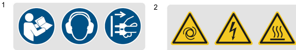
Fig. 1-1: Safety markings: 1 Mandatory sign - follow instructions, use hearing protection, pull out mains plug 2 warning signs - warning of automatic start-up, warning of electrical voltage, warning of hot surface
