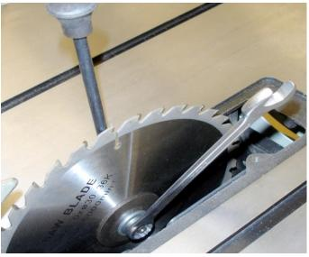
Use the 17mm spanner provided to unlock the nut on the saw spindle. Remove the nut, the washer, the saw flange and the blade.
