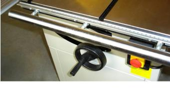
This double nut arrangement can be used to fine tune the alignment of the rip fence, so that it runs parallel to the blade.
