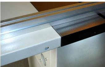
Using the long fence as a guide, level up the tables before tightening the bolts. Take the time to get this right as it is important to the accuracy of the saw.
