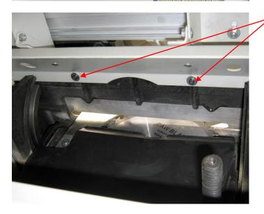
Next, using a 5mm hex key, loosen the two cap head bolts accessed through the side of the base under the sliding table.
