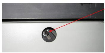
There is a similar Limit Stop for the 90 degree setting which is accessed through a hole at the rear of the machine.
