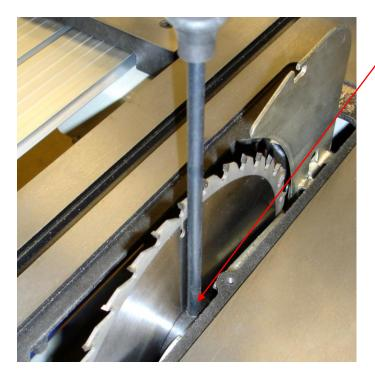
By hand, rotate the blade until the hole in the collar on the right hand side of the blade can be accessed.
