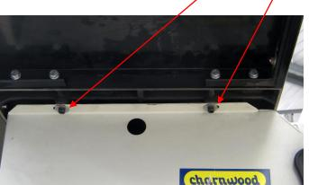
Loosen, but do not fully undo, the four M8 hex cap head bolts under the front and rear of the cast table using a 6mm hex key.
