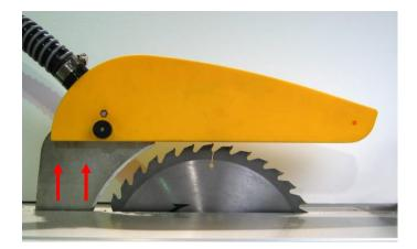
In order to keep the Crown Guard parallel to the table once the riving knife has been adjusted, a slight modification will need to be made to the slot.
