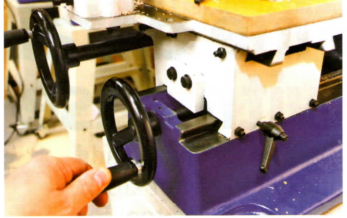
▲ The front to back adjustment is altered with this large wheel
