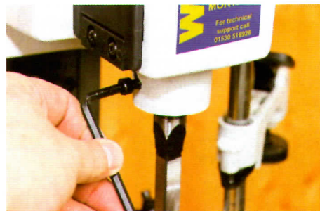
▲ You need a hex wrench to secure the chisel
