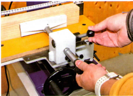
▲ A push in clamp, locked with the cam lever secures work firmly
