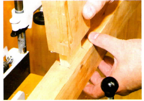
▲ The resulting mortises are clean and square
