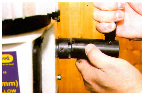
▲ The large plunge handle is easily repositioned to suit the work
