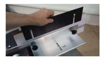
The shims vary in thickness and the set consists of 1 x 0.5mm, 2 x 1mm, 1 x 2mm. By using a combination of the shims, anything up to 4.5mm in 0.5mm increments can be set.
