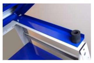
Attach the table side rails to the stand with two nuts & bolts and the rubber bumper bolts.
