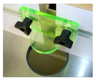
Take the two bolts that are fitted with tri-wing knobs and slide each bolt head into the channel in the front of the fence.
