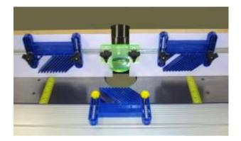
For safe and accurate routing, three feather boards have been supplied and these should be used whenever possible.
