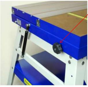
When closing the table top it will be necessary to secure it in the lowered position using the two table locking knobs.
