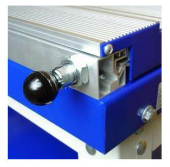
Attach the sliding carriage lock to the table by fitting a locking nut either side of the extrusion wall.
