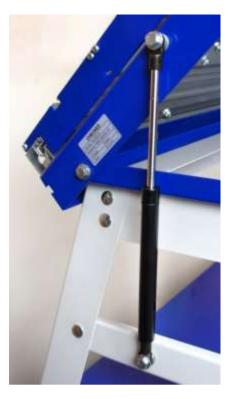
Note: Do not overtighten the NyLoc nuts as the spring needs to pivot.
