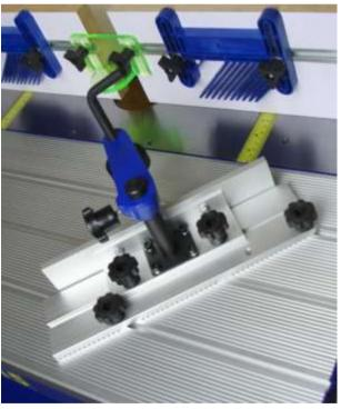
To set the Push Block to 45 degrees, remove the inner locking knob and reposition the bolt in the slot nearest to the fence.
