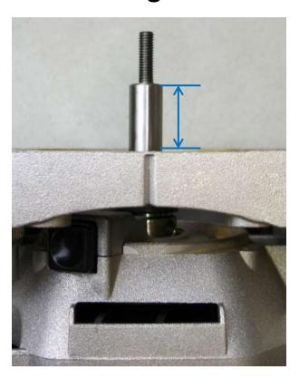
Consider removing the faceplate cover from the router base. Doing so will increase the maximum plunge depth by an amount equal to the baseplate thickness.
