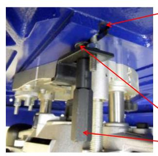
Slide both bolt heads into a slot in the underside of the table and position the mounting clamp on a convenient part of the router baseplate.
