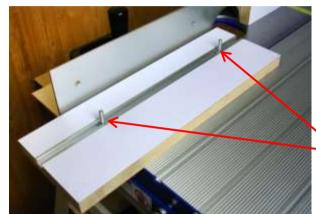
Slide the heads of two hex head bolts into the channel in the rear of the fence and fit them through the two holes in the fence carrier.
