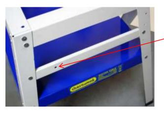
Fit a table lift support rail to either side of the table.
