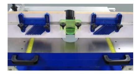
Undo the two fence fixing knobs, turn the fence through 180 degrees and then refit it using the two tapped holes nearest to the sliding table. This will often result in a more comfortable working position as the need to reach over the sliding table is eliminated.
