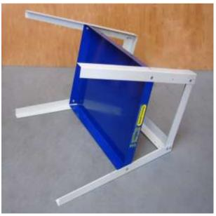
Lay the leg assembly on the floor and attach the middle shelf.
