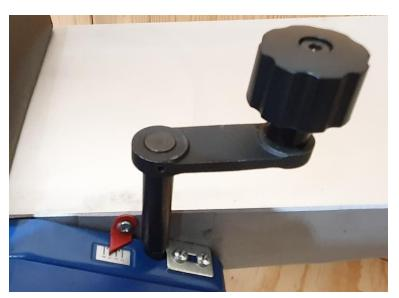
Use the crank handle to adjust the height of the thicknessing bed to match the work piece.
