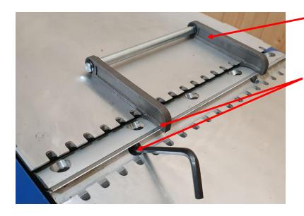
Place the knife height setting jig on the out-feed table with the curved section sitting over the knife and cutter block.
