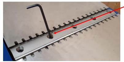
Using the 4mm allen key provided undo the 5 locking bolts (turn anticlockwise)
