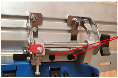
Fit the fence to the table, using the two M5 x 20mm cap head bolts and washers.
