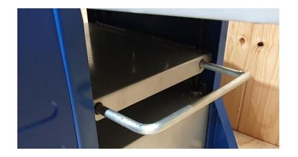
The out-feed end of the thicknesser bed has a pull-out support that can be extended to support the work piece as it emerges.
