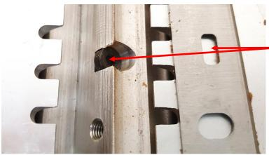
Place the new knife into the cutter block.
