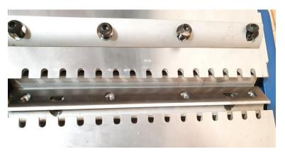
Once the new knife is in place, refit the locking bar.
