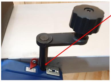
Fit the crank handle onto the shaft located at the side of the infeed table.
