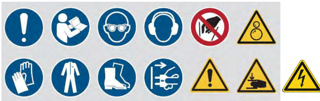
Fig.1-2: Safety signs - Prohibition sign: No reaching! | Mandatory signs: Observe instructions for use, unplug, wear eye protection, wear hearing protection, wear foot protection, wear hand protection, wear protective clothing | Warning signs: Warning of hand injuries, warning of electrical voltage, warning of counter-rotating rollers!
