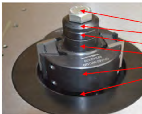
Fig.8-8: Engaging the spindle lock
