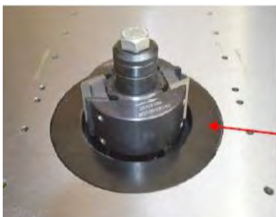
Fig.8-6: Mounting a knife shaft
