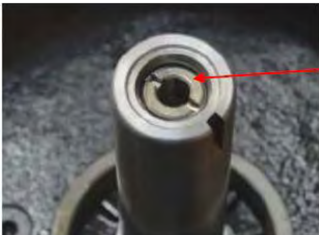
Fig.8-5: Remove retaining ring
