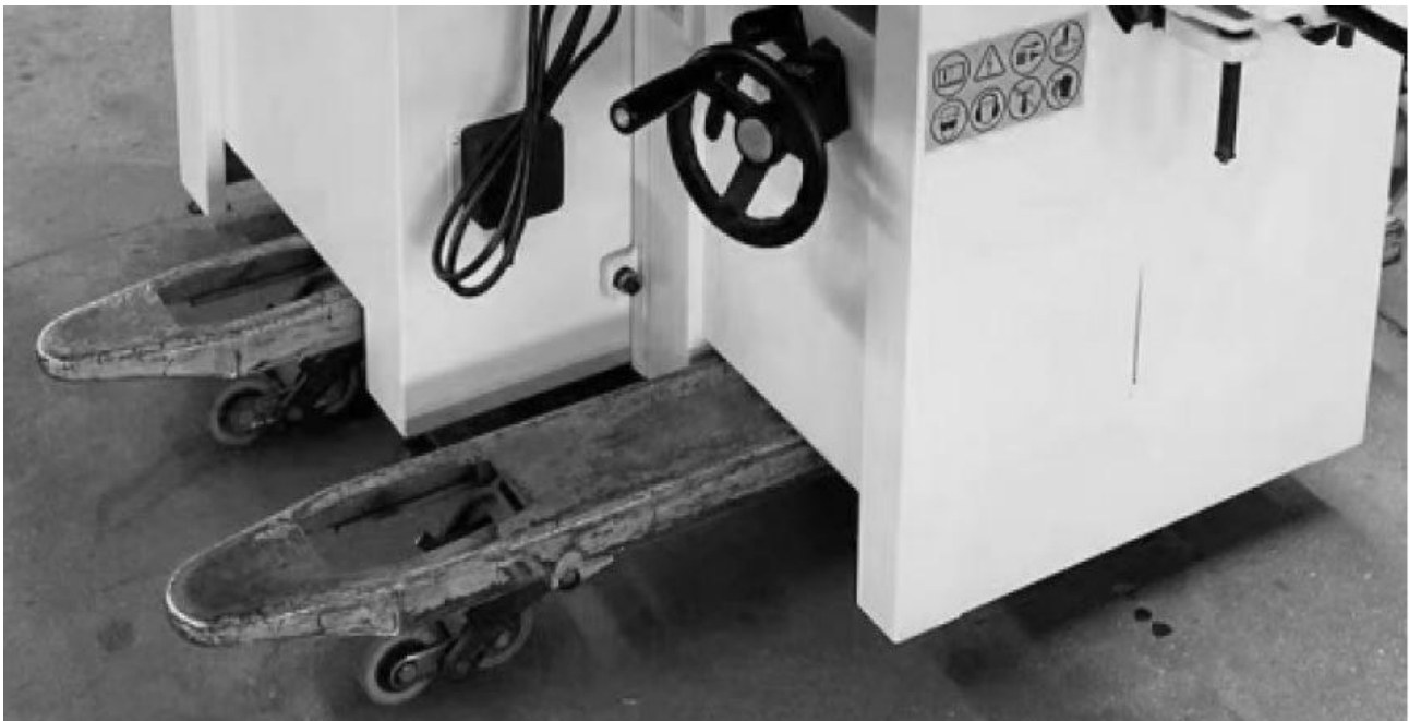
Fig.3-1: Transporting the machine with a pallet truck or forklift
