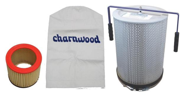
A typical hobby level high volume dust extractor will be supplied with a cloth filter, with a rating of 5 microns. That means it will filter out 99% of dust particles at 5 micron size or bigger. It will also trap some smaller particles too but to a lesser level, so at 1 micron it might only be 50%.
