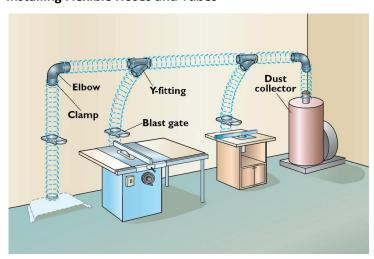
Flexible hoses are sold by the metre. Design your network and measure up the length of hose you need. Buy the hose in a single length and then cut it down yourself, just using a craft knife and a pair of side cutter pliers.
