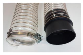
Imagine the end of the hose is the nut and the quick push connector is a bolt, which way would you turn it to screw it in. Hoses are available in both right handed (the normal way!) and left handed versions from different manufacturers. Hoses supplied with machines (foreign made) are most often left handed. Charnwood hose, sold by the metre, is UK made and has a right handed thread.
