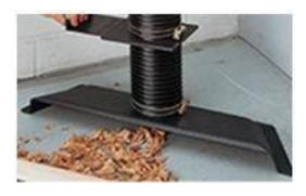
The other option is to bring the dust to the extractor by using a floor mount dust hood. The dust hood is connected to a hose branch from the extractor. Turn the extractor on and use a brush to sweep the chips into the mouth of the dust hood.
