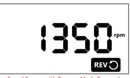
Speed Screen with Reverse Mode Engaged
