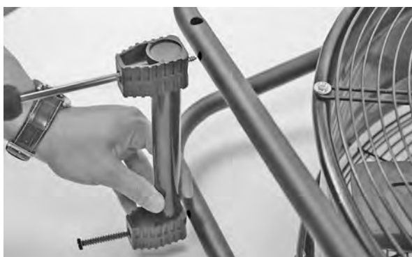
Fig. 10: Connect the foot element to the base frame
