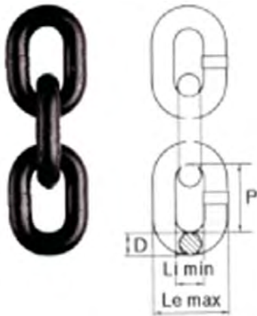
Fig. 4: Dimension of the chain
