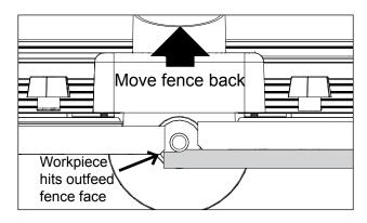
If the bit gouges the scrap at the trailing edge, the fence is too far back, and you're removing too much material. Use the micro-adjuster to move the fence forward.
