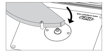
**WARNING** Use the starting pin when routing along curved edges and only with router bits that have a guide bearing. When routing along straight edges, always use the fence.
