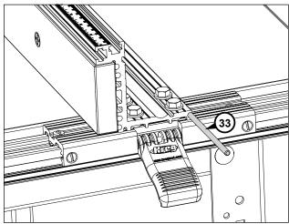
To store the jointing rods (33), slide them into the round channel at the back edge of the fence extrusion base flange. (See **Jointing** under the section **Using Your Router Table Fence**.)
