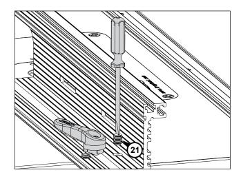
Thread two set screws (21) into the holes flanking the ¼-turn handle. You'll use these screws to square the fence. (See the section Align and square the fence.)
