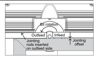
Use a scrap piece of wood to test the setup. If you feed the scrap past the bit and it runs into the leading end of the outfeed fence face, the fence is too far forward and you're not removing enough material. Use the micro-adjuster to move the fence back.
