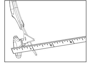
Before installing the self-adhesive measuring tape, make sure the shallow groove in the top of the fence is clean and dry. To hold the miter gauge steady while you install the tape, place the miter gauge in the saw miter-gauge slot. Cut the tape at the 1" mark and the 25" mark using sturdy scissors or metal snips.
