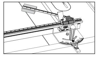
Make a test cut to confirm the 3" length. Adjust the cursor position as necessary and make another test cut.
