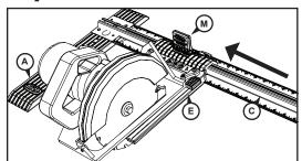
With your saw clamped to the sled (E), raise the handle (M) to the upright position and slide the sled onto the rail (C), inserting the wedge (L) into the rail channel. The saw and the edge guide (A) should extend from the same edge of the rail.
