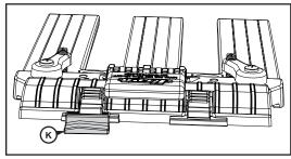
There are two positions on the sled for the cursor (K) that correspond to the two sled slots. Position the cursor in the holder in front of the saw blade. To switch cursor position, press down on the holder lock, slide the cursor out of the holder and reinstall it in the other holder.
