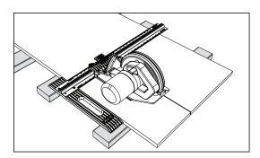
5) Connect your saw to power. With one hand on the edge guide and the other holding the saw, press the edge guide against the edge of your workpiece and make your cut, moving the edge guide and saw forward at the same speed throughout the entire cut. Allow the saw blade to come to a complete stop before lifting the Rip-Cut™ from the workpiece.
