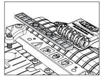
The filler strip (D) on the sled (E) is shipped with the angled ribs facing up. These ribs support a saw base with an angled leading edge, keeping the saw base flat on the sled when the set screws (F) in the base-plate clamps (G) are tightened. For a saw base with a flat leading edge, lift the filler strip from the sled recess with the tip of a screwdriver, turn it over to expose the flat face, and press it into the recess.
