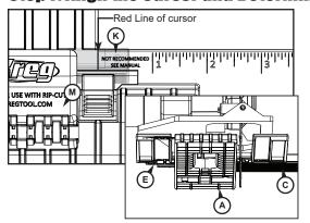
Rotate the saw blade guard up and slide the sled **(E)** along the rail **(C)** until the blade just touches the edge guide **(A)**. Lock the sled in place by pressing down on the handle **(M)**. The handle does not need to be completely horizontal to lock securely. Press down on the cursor lock and align the red cursor **(K)** with the zero mark on the rail scale. The minimum safe cut may be greater than 1".
