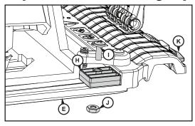
The indexing stop (H) allows you to remove the saw from the sled assembly and then re-mount it in exactly the same position. Place the indexing stop against the side of the saw base on the same side as the cursor (K) and secure it to the sled (E) with the machine screw (I) and nut (J). For maximum positioning flexibility, the sled is slotted and the indexing stop rotates 180°.
