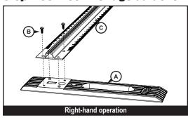
Remove the clear tape covering the recess in the edge guide (A), remove the two self-tapping screws (B), and use them to secure the edge guide to the rail (C). Orient the edge guide for right-hand or left-hand operation as shown.
