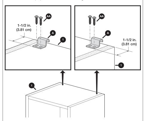
Note The top of the cabinet must be flush with the sides. If it isn't, cut a scrap piece of plywood or lumber (1) the correct thickness to make it flush and attach securely to the top. The cabinet top must also be 1/2 in. (1.27 cm) thick or thicker. If the cabinet is 24 in. (60.96 cm) wide or smaller, two brackets should be sufficient. More brackets may be needed if the cabinet is wider, taller, or deeper than a typical wall cabinet.
